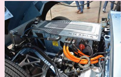
Retrofitted Battery Electric drivetrain
