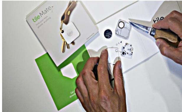
A sawn apart and disassembled Tile, revealing the printed circuit board (PCB) with a standard battery, being soldered to the printed circuit board. Image: Thomas Nyström
